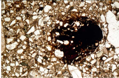
Fig. 175: Photomicrograph of M719594B (wall ditch 704392/707151, House 59); wood char fragment showing iron staining and embedded silt and fine sand. PPL, frame width is ~0.90mm.
