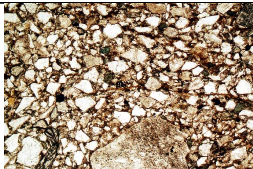
Fig. 264: Photomicrograph of M722795B (Pit house 711333, lower Layer 2); compact partially waterlaid loamy fine sands, with detrital organic matter. PPL, frame width is ~2.38mm.
