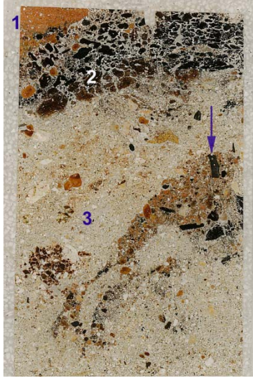
Fig. 34: Scan of M48126 (Furnace 246798); Layer 1 – rubefied (moderately strongly heated) mud-plastered daub furnace wall (Figs 35-36); Layer 2: possible trample of iron stained charcoal, char, slag-like materials and iron fragments (Figs 37-40); Layer 3: steeply sloping backfills of previous iron working activity and including possible hammerscale (arrow; Figs 41-42). Frame width is 50mm.
