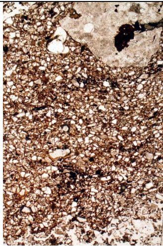
Fig. 198: Photomicrograph of M722099 (Furnace 707119, House 60); silt loam mud plastered constructed furnace material with embedded heated rock fragment of presumed Layer 3 origin. PPL, frame height is ~4.62mm.
