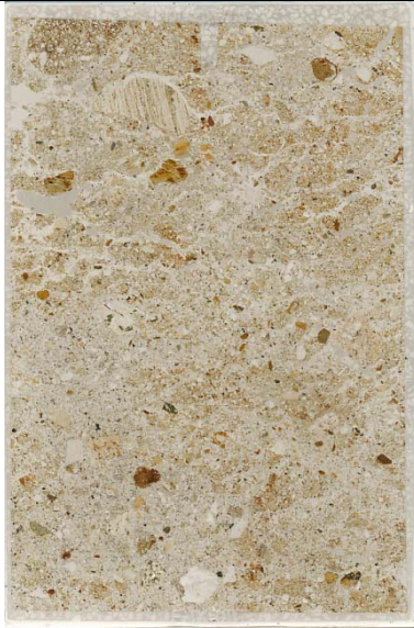
Fig. 65: Scan of M62671B (Furnace 44562, House 69, Layers 2-3); lower part of furnace constructed by mud plastering using a fine sandy silt loam – here showing no evident effects of heating, but with an apparent lenticular microstructure resulting from frost action. Frame width is ~50mm.
