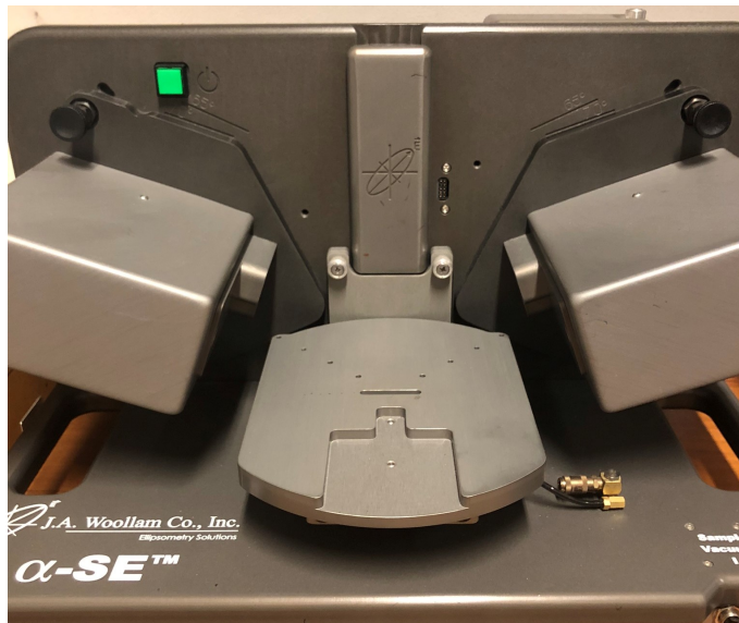
Figure 3.6: J.A. Woollam Ellipsometer Setup showing the light source, detector and sample stage.
