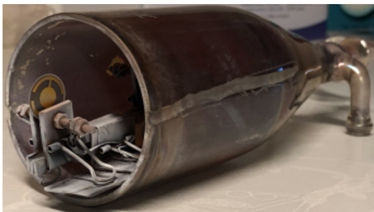
Figure 3.4: QCM setup showing the Quartz crystal holder setup located at the center of the reaction chamber, the QCR sensor nearest the exhaust.
