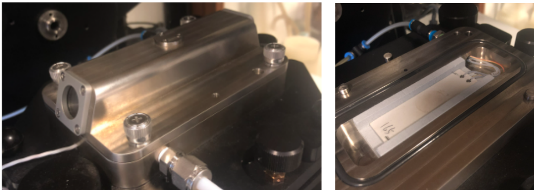
Figure 3.7: J.A. Woollam Ellipsometer setup showing the closed (left) and open (right) environmental chamber.
