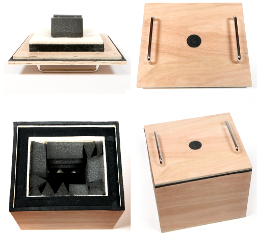
Figure 1: Fully constructed mini acoustic chamber. (Top left) Side view of the bottom part of the top cover. (Top right) Top view of the top cover. (Bottom left) Inside of the chamber. (Bottom right) Fully assembled chamber. The two handles are used to lift open the top cover. The round hole in the center for accessing the chamber for measurement (e.g., microphone) and observation (e.g., digital microscope)
