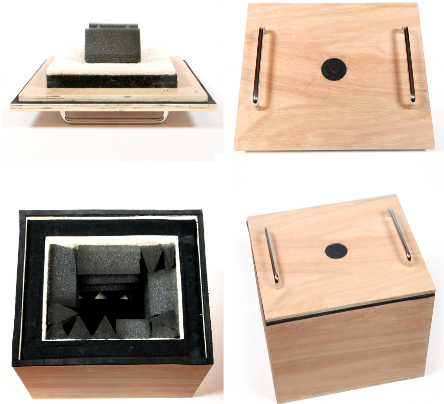
Figure 4.9: A fully constructed mini acoustic chamber. (Top left) Side view of the bottom part of the top cover. (Top right) Top view of the top cover. (Bottom left) Inside the chamber. (Bottom right) Fully assembled chamber. The two handles are used to lift open the top cover. The round hole in the centre is for accessing the chamber for measurement (e.g., microphone) and observation (e.g., digital microscope).
