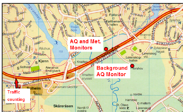
Figure 2.1a. Map of the Nordbysletta area and the main roadway. Locations of monitoring stations for air quality, meteorology and traffic counting are indicated in the figure by the red dots and red arrow.
