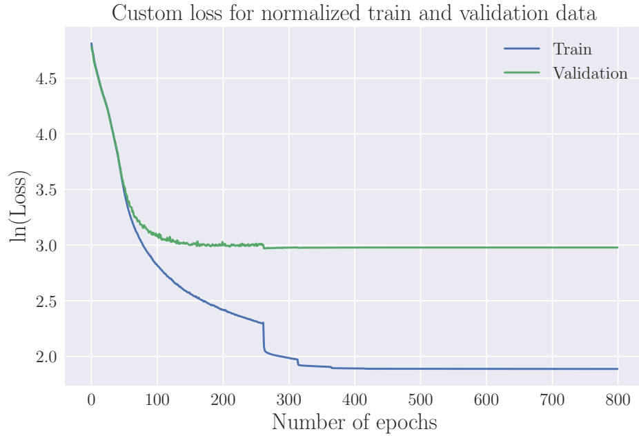
Figure 9.5: Training- and validation loss for the CNN, predicting two current dipole sources, as function of epochs.
