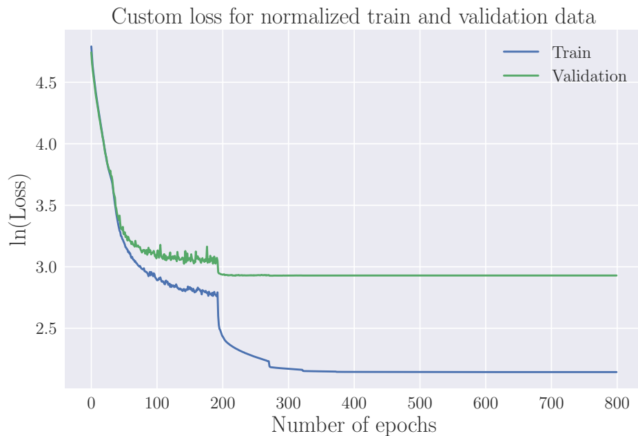
Figure 9.2: Training and validation loss for the FCNN, predicting two current dipole sources, as function of epochs.
