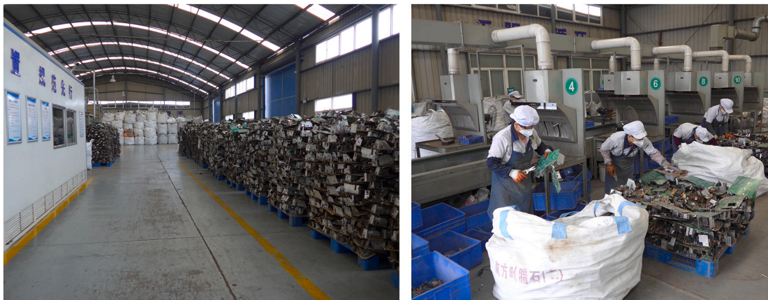
Fig. 5. Recycling of PCBs from computers. Left: Storage on the right and high-temperature separation area on the left. Right: Manual dismantling.
