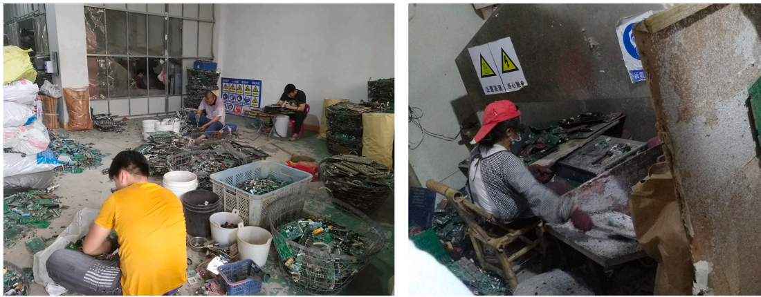
Fig. 3. Recycling of PCBs in Guiyu. Left: Manual dismantling. Right: High-temperature separation of components.
