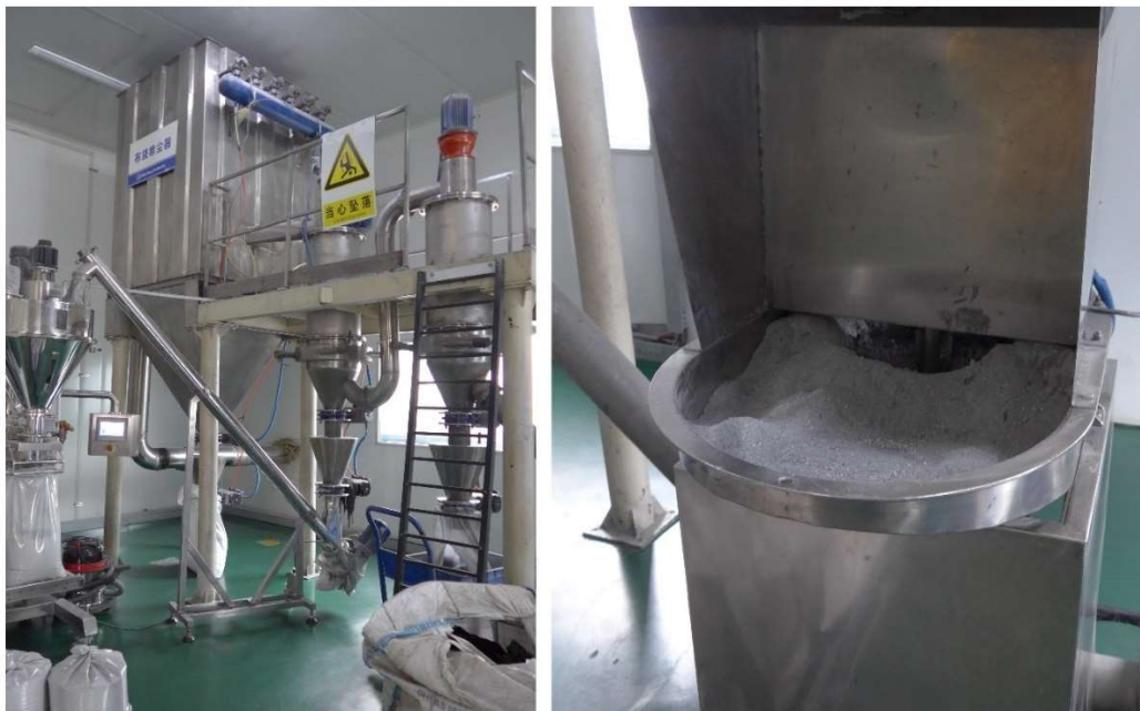
Figure 20. Recycling of CRTs from televisions in a company in China. Left: Machine for the mechanical treatment. Right: Refining of lead from the recycling process.
