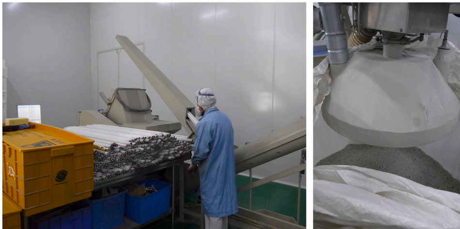
Fig. 6. Recycling of fluorescent lamps. Left: Insertion of lamps into the machine. Right: Extraction of glass from the recycling process.
