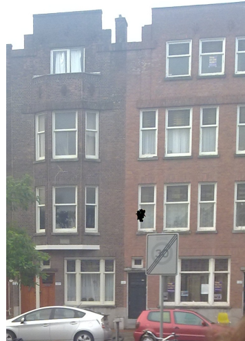
Figure 3.10: picture of a damaged image sensor, credit: [23, Vera de Kok], license CC BY-SA 3.0
