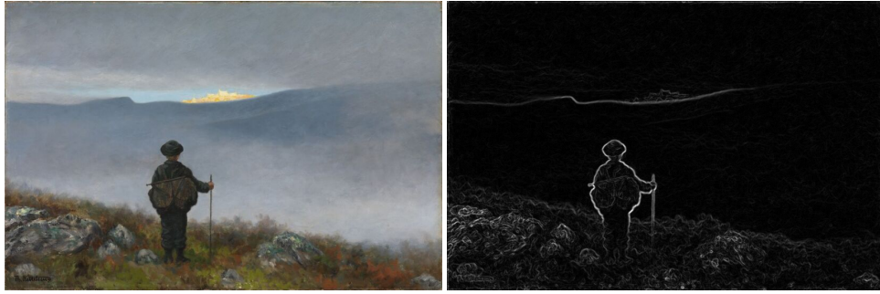
Figure 2.1: The image to the right show the gradient magnitude after the Sobel filter has been applied. The image to the left show the original image before the transformation. (Nasjonalnuseet [40])
