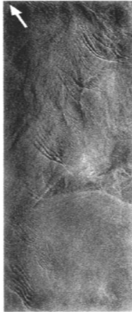
Figure 1.5: ERS-1 SAR image ( 30 \times 100 km) of internal waves outside Andøya, Norway, where the white arrow indicates the North direction. A total of 8 wave trains, with an average distance of 10.8 km between the trains, can be seen propagating against the coastal current. Image adapted from Dokken et al. 2001, with permission from Wiley.
