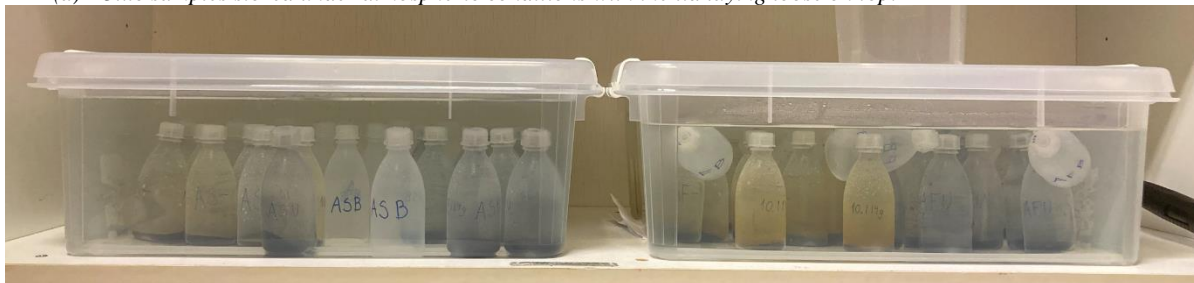
(b) Low-oxygen samples stored in boxes filled with water. Photo was taken before freshwater blanks got glass plates to avoid floating.
