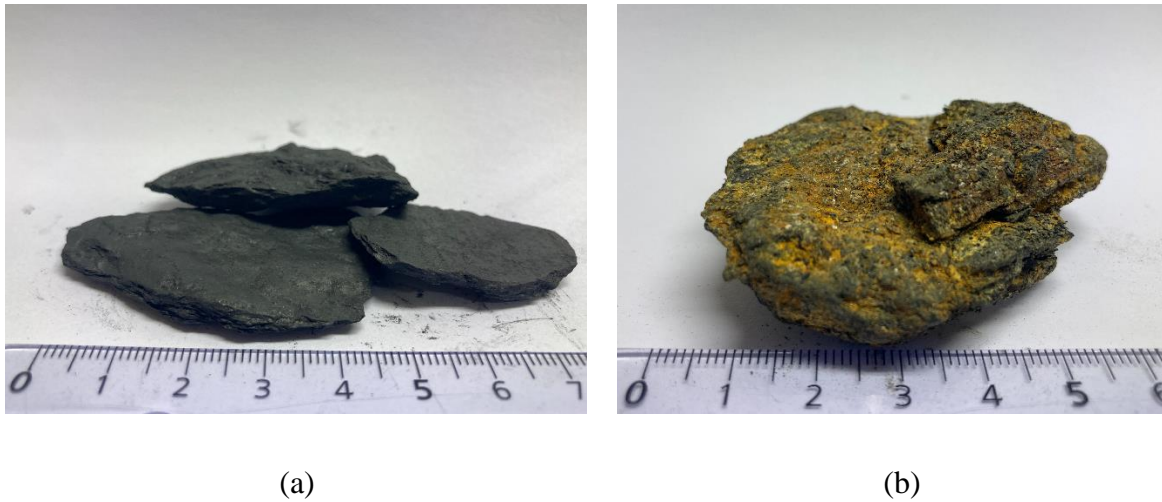
Figure 4: Figure (a) shows unweathered alum shale from Kleggerud with its characteristic black colour. Figure (b) shows weathered alum shale deposited at Taraldrud with secondary sulphate minerals on the surface.
