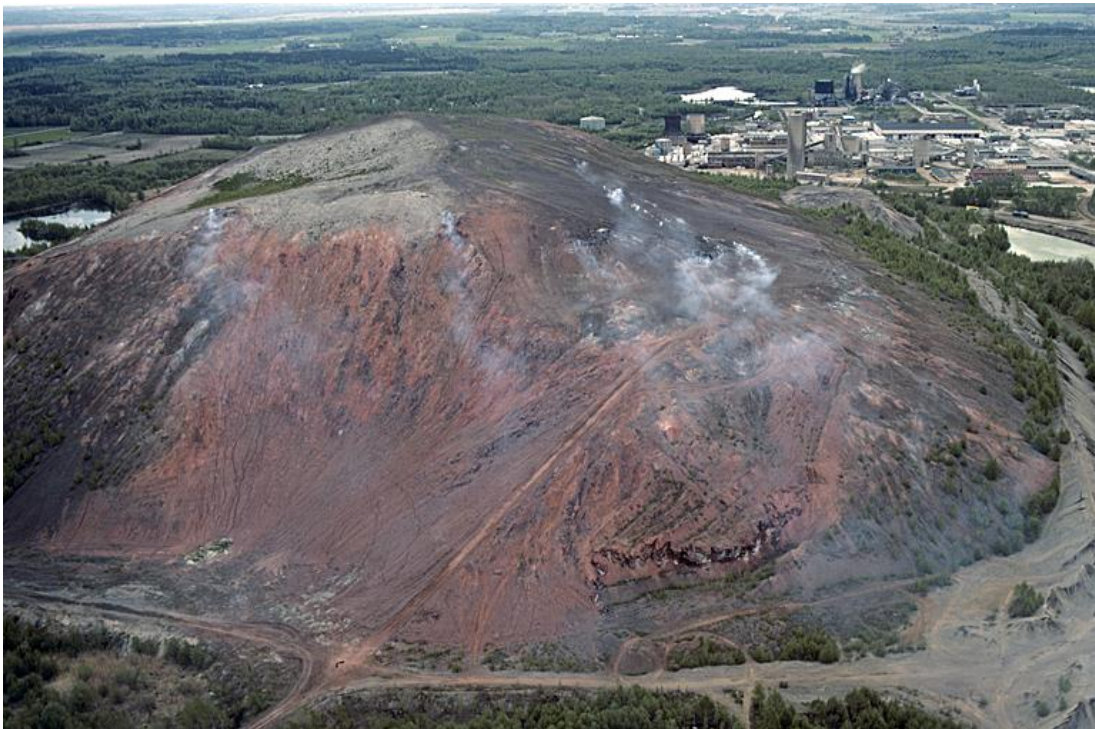
Figure 6: Kvarntorp, Sweden: Burning pile of residual masses from oil extraction of alum shale. The photo is probably from the mid-1970s. (Photo: Pål-Nils Nilsson).
