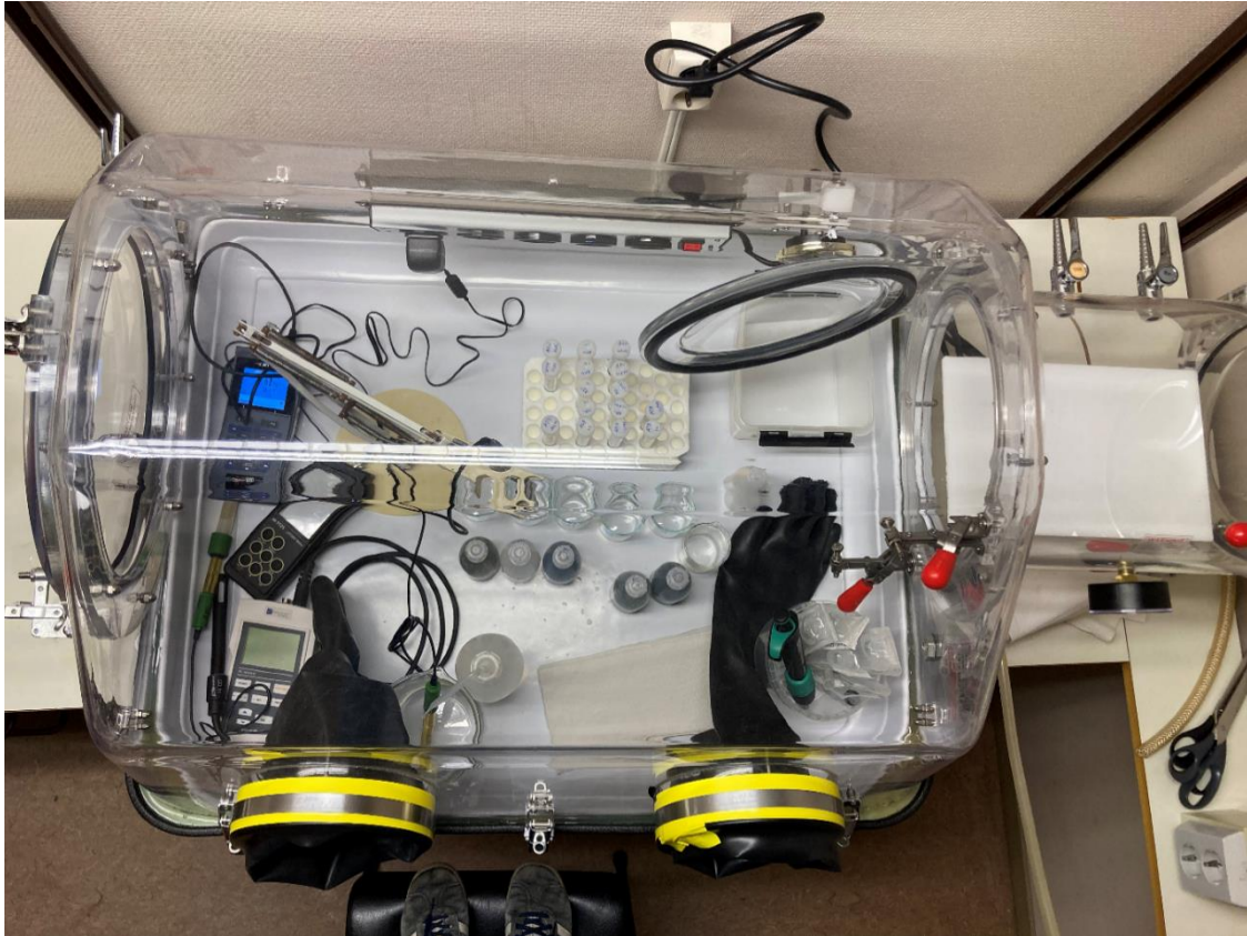
Figure 15: Sampling of low-oxygen samples in the glove box.
