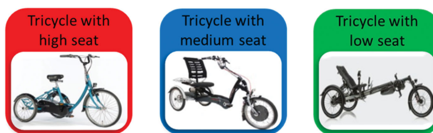
Figure 1. Images of the three tricycle categories. High seat = > 70 cm, medium seat = 57–63 cm and low seat = < 57 cm.
