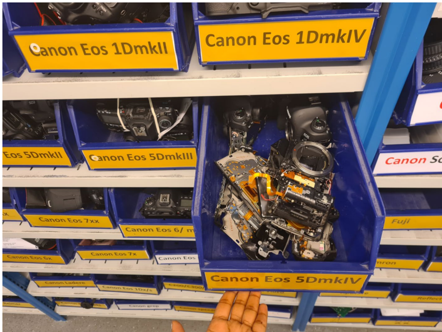
Fig. 4 Cannibalised spare parts from photo cameras
