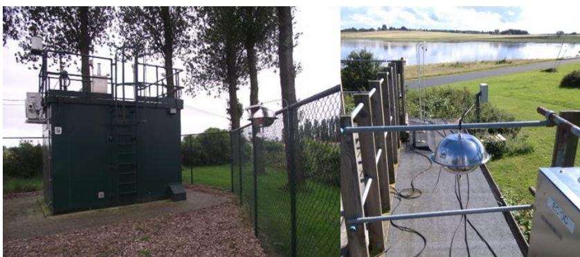
Figure SI-1.2. Passive air samplers deployed in close connection to existing monitoring stations, illustrated by site 4 (Houtem) in Belgium (photo: E. Adriaenssens) and site 13 (Risoe) in Denmark (photo: T. Ellermann).
