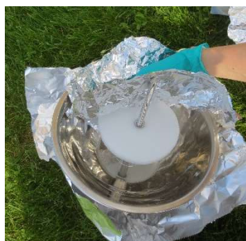
Figure SI-1.2: Mounting the PUF disk
