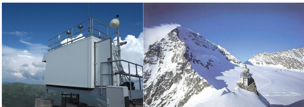
Figure SI-1.4b. Site 70 (Chopok, Slovakia) and site 86 (Jungfrauoch, Switzerland), situated at high altitudes (2008 and 3578 m.a.s.l. respectively), resulting in both low temperatures and high exposure to wind (and hence elevated sampling rates).
