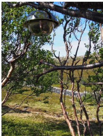
Figure SI-1.3. A passive air sampler deployed in field (site 20).
