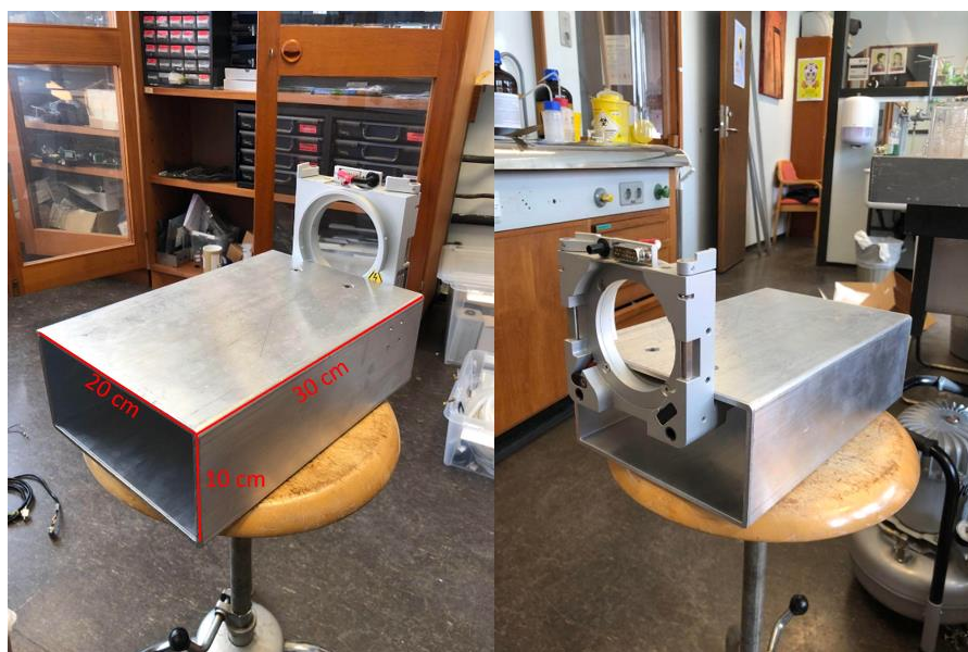
Figure 30. The pictures show the open-ended aluminum cuboid shape used as a base for the ion source. A Nanospray flex interface was taken apart and mounted onto the base for easy mantling and dismantling of the ion source onto the mass spectrometer.
