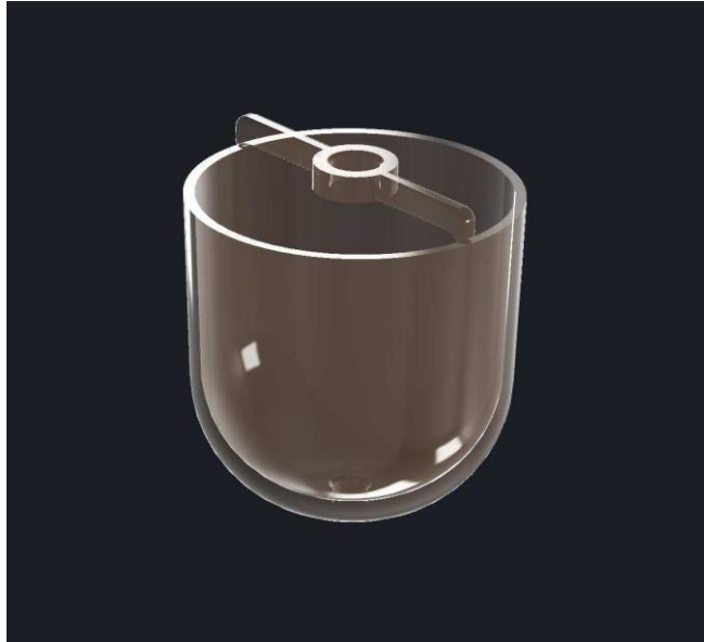
Figure 17. Model of an etching cup made using 3D-printing. Made by Inge Mikalsen. The bridge arcs over the opening of the cup and contains an orifice that aligns with the bottom hole, both through which the capillary is threaded during etching. The cup measures 5,2 mm in height, and 4,9 mm at its widest diameter. The cups are made using the Clear Resin from Formlabs.,
