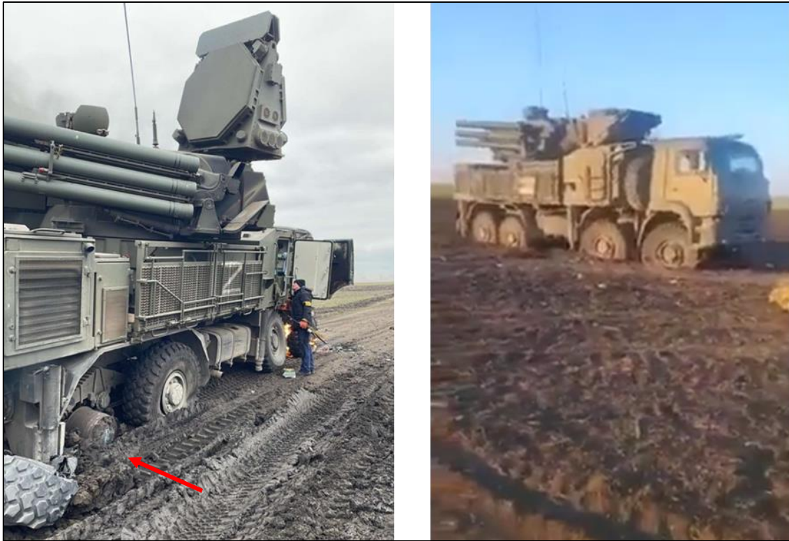
Picture 6: Russian Pantsir-S1 SAM vehicles stuck in the mud after its tires burst 163
