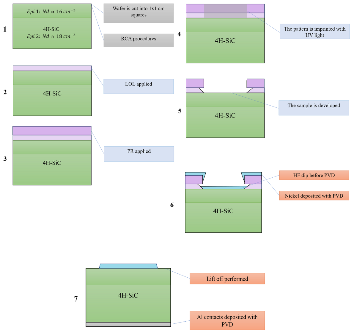
Figure 23 4H-SiC Schottky diode fabrication schematic.
