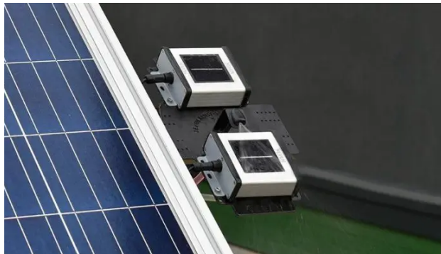
Figure 2.12: A soiling station showing an automated periodical cleaning functionality for the lower cell. The figure was adapted from Barnes [57].
