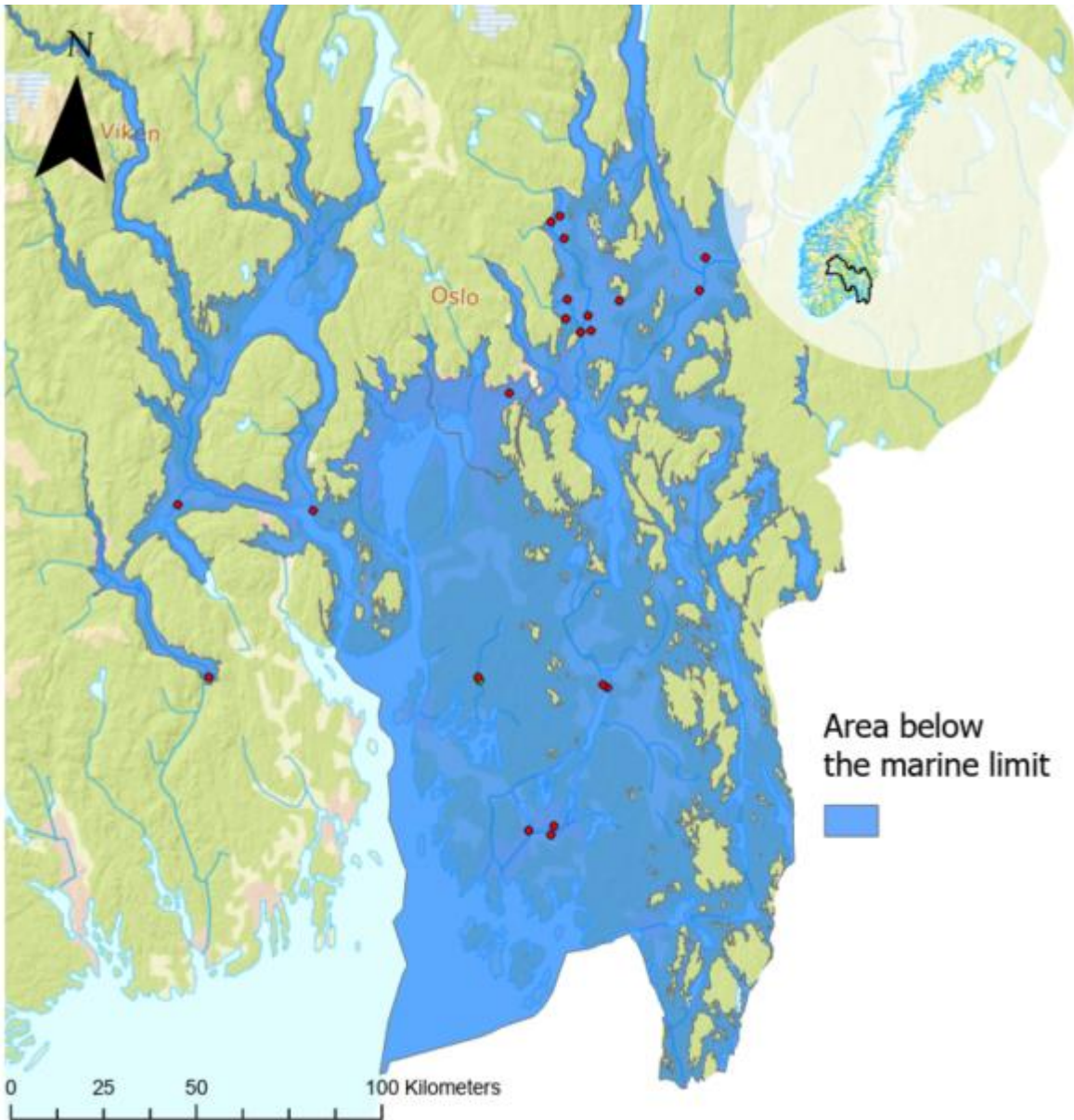
Figure 8 - Map illustrating which part of the study area (Figure 7) is below the marine limit, with red dots indicating quick clay landslides used in the analysis. Background map: Topografisk Norgeskart 4.
