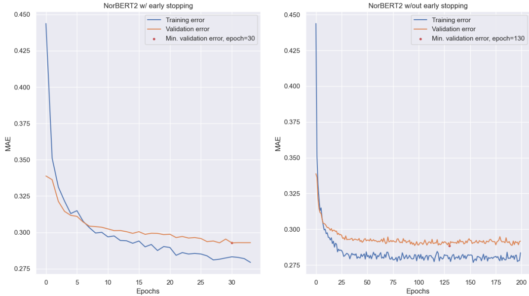
Figure 4.1: Mean training and validation errors for each epoch during training of NorBERT 2 with and without early stopping. The learning rate in these experiments was 0.001 and the batch size chosen was 256. The test error yielded with and without early stopping were 0.2764 and 0.2737 respectively.
