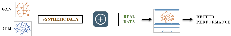
Figure 3.1: Deep generative models (GAN and DDM) can be used to synthesize high quality echocardiography images, both 2D and 3D. These images can be then used to train and improve DL algorithms.
