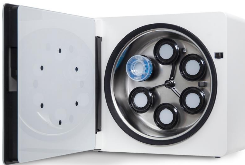
Figure 6. The CelVivo rotational 3D cell culture system used to generate 3D cell spheroids (172).
