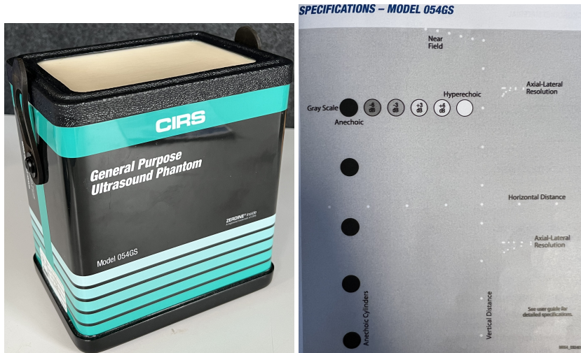
Figure 2.8: The tissue-mimicking phantom 054GS from CIRS embedded with several cysts and wire targets.
