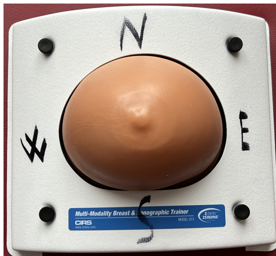
Figure 2.9: The Multi-Modality Breast Biopsy and Sonographic Trainer M073 from CIRS. The phantom accurately mimics the heterogeneous appearance of breast tissue under ultrasound, mammography, and MRI. It has cystic and dense lesions with 100-300 micron microcalcifications.
