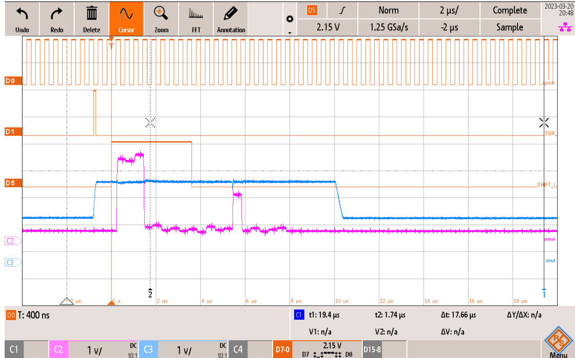
Figure 6.7: After adjusting the hold signal to hold the output signal aout for a longer time, all the signals are multiplexed out of amux and the ADC samples the correct output values.
