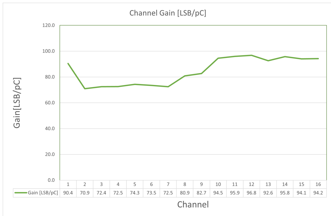
Figure 6.9: Measurement shows gain variation between all channels
