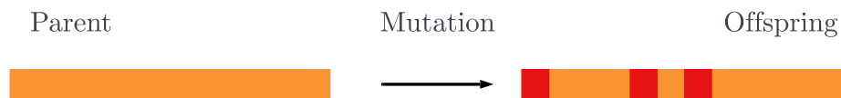
(b) Mutation of a single cloned parent results in an offspring containing the genes of the parent with one or more genes modified. Modified genes are shown in red.
