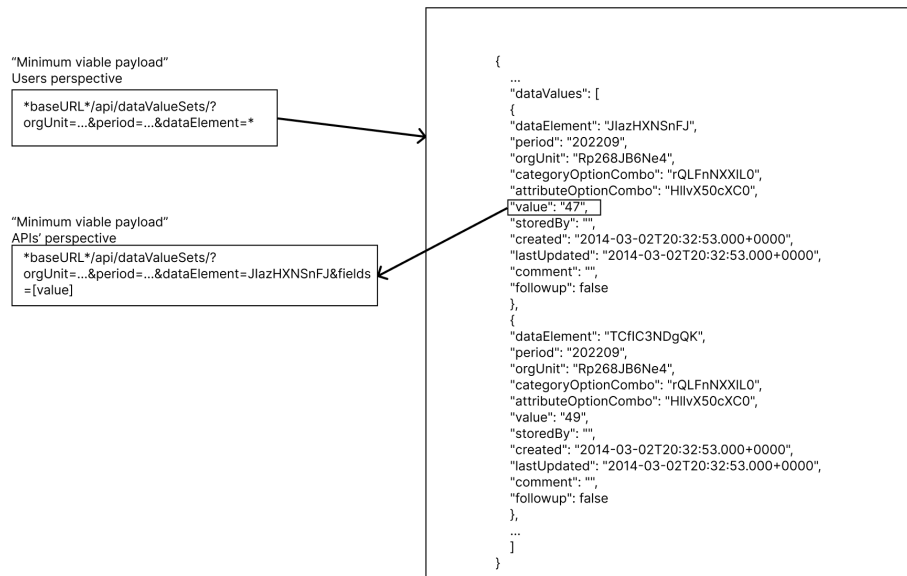
Figure 25: Perspectives on "Minimum viable payload" Presentation of the different perspectives on "Minimum viable payload". Note that the example is purely for illustration and is not necessarily an accurate request/response.
