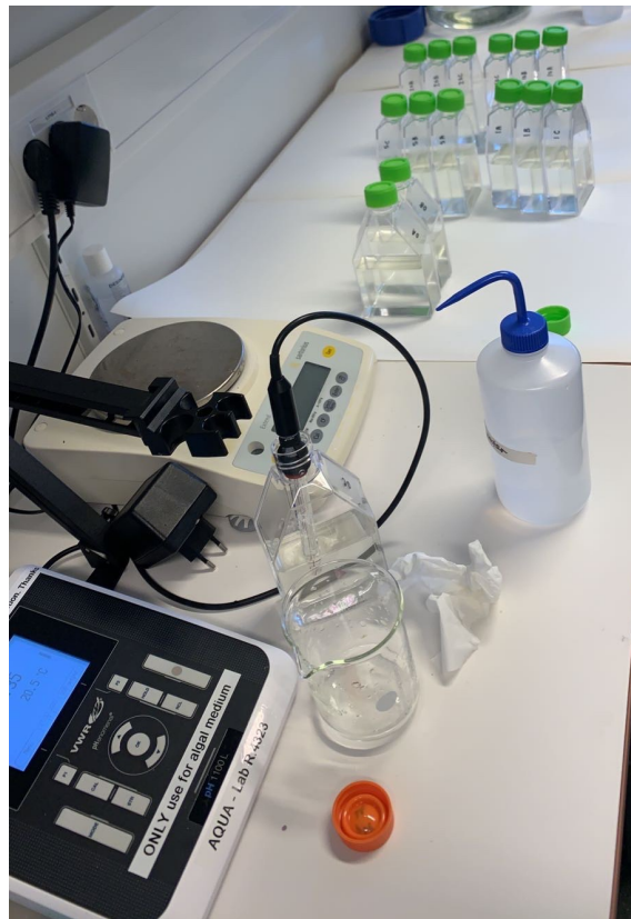
Figure S2. Measuring the pH of each algal concentration bottle prior to adding grazing copepods during the toxicity induction experiment. Between each measurement, the sensor was rinsed with filtered seawater with a corresponding PSU.
