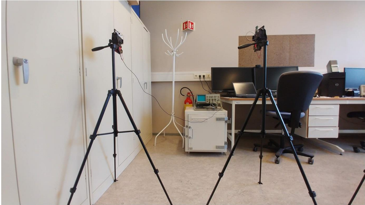
Figure 22: Setup for measuring ToF between a transmitter (to the left) and a receiver (to the right).
