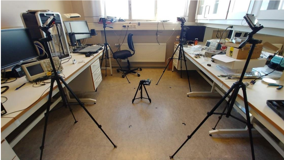
Figure 25: Setup of the ultrasonic positioning system. Four anchor nodes (transmitters) are placed at a height pointing their transducers at the center of the positioning area, and the receiver points its microphone towards the ceiling. The anchor nodes form a 3D space where the direct line-of-sight ultrasonic pulse can be detected and used for position estimation of the receiving node.
