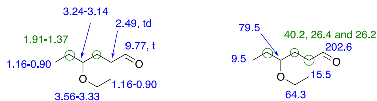
Figure 28 Assignment of 1 H NMR (left) and 13 C NMR (right) signals for protected aldehyde 3 .
