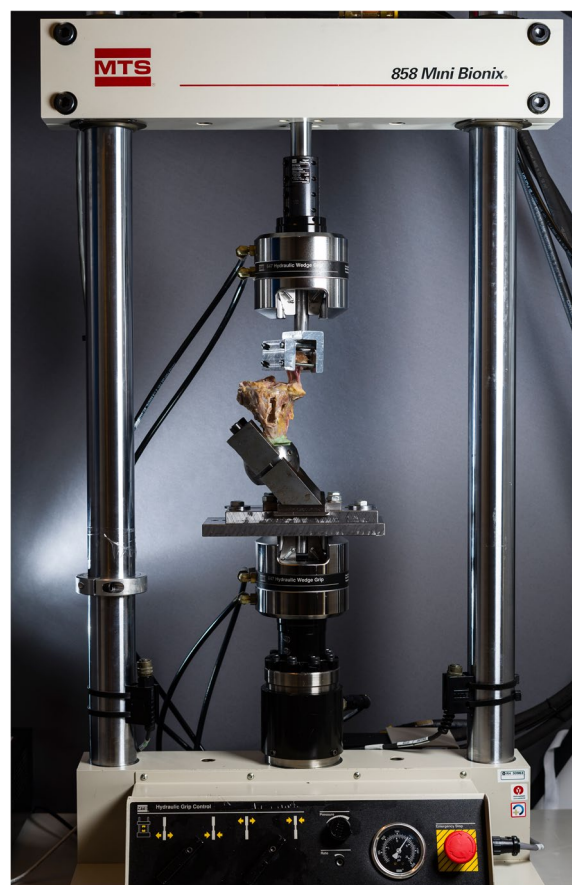
Fig. 2 Biomechanical setup. Biomechanical setup in the MTS ® machine. The tibia is fixed with polymethylmethacrylate and screws to a steel tube and the femoral bone block to a metal clamp
