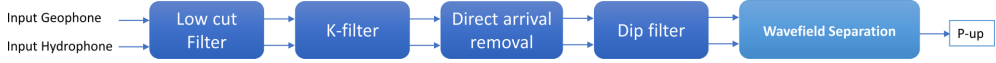
FIGURE 10 Different pre-processing steps before applying the dual-sensor wavefield separation to the field data example of 3320 shots.
