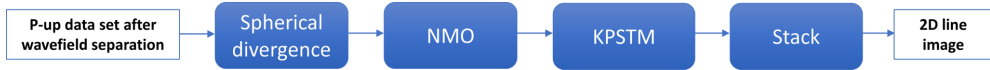
FIGURE 12 Main steps of the seismic processing workflow to generate a 2D line image after applying the dual-sensor wavefield separation process using the FK and the WSPDL methods.
