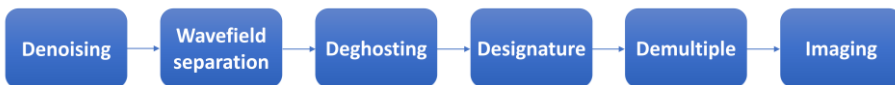
Figure 1.3: A simple processing workflow after acquisition including imaging. First data are denoised and separated into up- and down-going parts of the wavefield. Then the deghosting, designature, and demultiple processes remove the effects of the source signature and the sea surface. Finally, the data are migrated to obtain an image of the subsurface.
