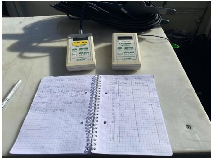
Figure 2.3. Illustration of setup during light intensity measuring. Two light meters were used: one for the underwater quantum sensor (left) and the other for the quantum sensor on deck (right). Average measurements for each depth interval were recorded from each light meter.
