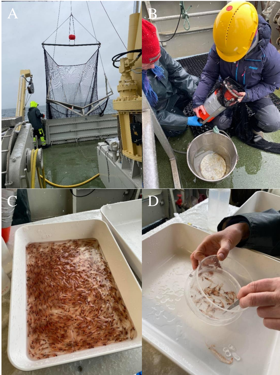
Figure 2.5. A: IKMT retrieved after sampling. Note the depth sensor attached (red brick). B: 500 mL bucket at the end of the IKMT with the biological sample. C: The catch after sampling with IKMT. Notice the dominance of M. norvegica . D: Sorting the biological sample. Note the jellyfish and the individual of Pasiphaea sp.
