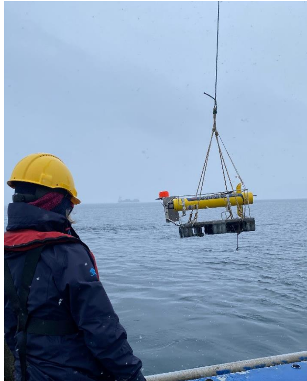
Figure 2.6. Image of WBAT seafloor rig during deployment. Consists of a crate with weights attached, the transceiver (yellow tube) and transducer (orange cap).
