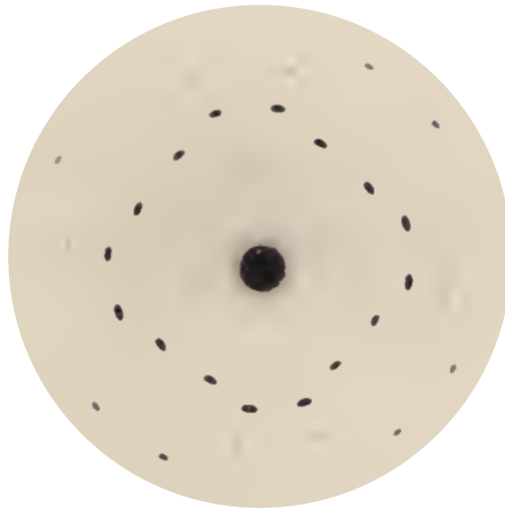
Figure 1.2: One of the first diffraction patterns from x-ray scattering of ZnS, as reported in the publication by Max von Laues group in 1912 [9] (public domain).
