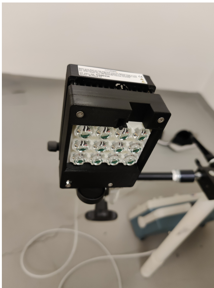
Figure 34: Close up of the LED lamp used as a light source, mounted with 15° optics
