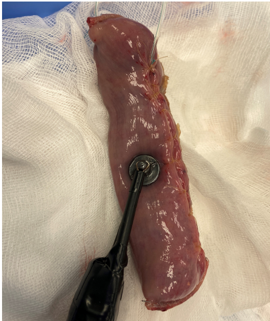
Figure 2.5: Experimental setup for bioimpedance measurements on the human small intestine.
