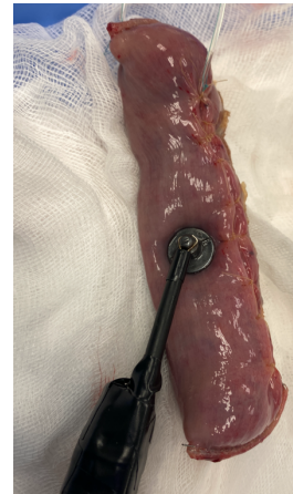
Figure 1: Experiment set-up. Human intestine sample under measurement.
