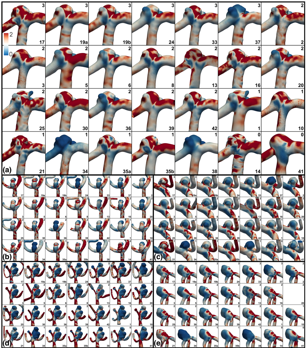
FIGURE 6. Variability of normalized WSS*, with (a–e) showing Cases 1–5. WSS* values are plotted from 0 to 2 using the colour scale shown in the top left panels, where WSS* = 1 corresponds to the nominal parent artery value. Experience levels and team numbers are shown in each panel, as explained in the caption of Fig. 2.
