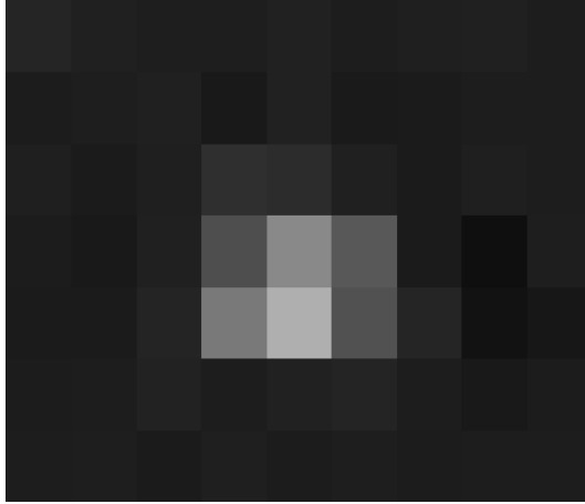
Figure 5: Typical particle image in our experiments. Each square equals to one pixel in the original image.
