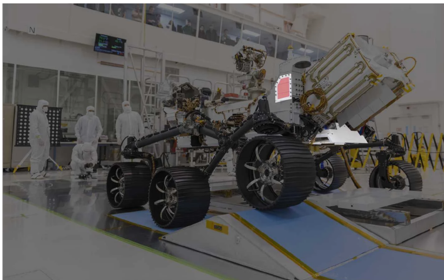
Figure 1.1: Photo taken during Assembly, Test, and Launch Operations (ATLO) at NASA Jet Propulsion Laboratory (JPL), highlighting where RIMFAX is mounted on the Perseverance rover spacecraft. Location of electronics box within left aft tower (red highlight) and antenna at lower aft. Figure from Hamran et al. (2020). Image credit: NASA/JPL-Caltech.
