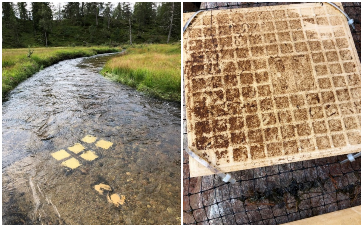
Figure 8. Ceramic tiles were our standardized substrate for biofilm growth in the control and impacted river reaches (Photos: Lorenzo Pin).
