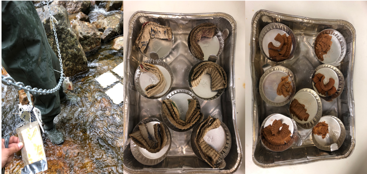
Figure 9. Wettex stripes were used as proxy to measure the organic matter breakdown in the impacted and unimpacted reaches. After the exposure period the dry weights were measured and then the samples were burned to calculate the Ash Free Dry Weight.
