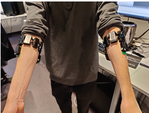
Figure 6. Placement of the EMG sensors on the arms of the guitarists. Two Delsys EMG sensors were placed on each side of the arm, right below the Myo armbands.
