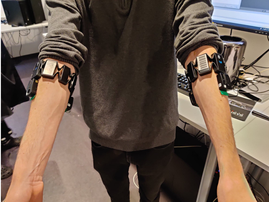
Figure 3.5: Placement of the EMG sensors on the arms of the guitarists. Two delys EMG sensors were placed on each side of the arm, right below the Myo armbands.
