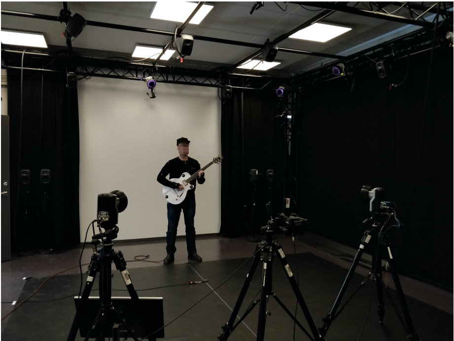
Figure 3.4: A participant during the recording session. Motion capture cameras can be seen hanging in the ceiling rig behind, and on stands in front of, the performer. The monitor with instructions can be seen below the front left motion capture camera.
