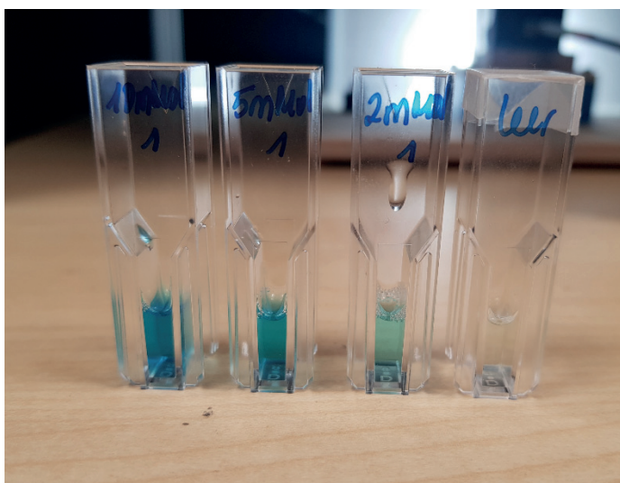
Figure 5: Illustration of the reaction between formate and formate oxidase (FOX) enzyme that gives a colour change to blue after 5 minutes. From left; formate 10 mmol/L; 5 mmol/L; 2 mmol/L and control (without formate).
