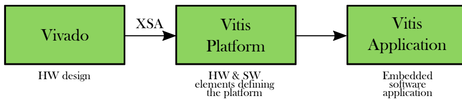
Figure 5.4: Diagram illustrating the design flow of the chip control using an on-board FPGA on the PYNQ-Z1 board.
