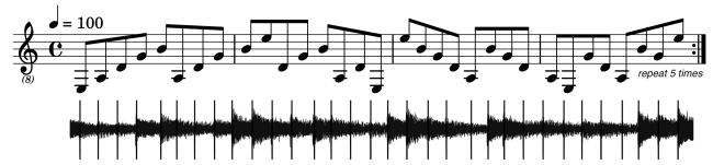
Figure 5: Top – The music used to measure Professor Plucky’s timing. Bottom – Waveform of Professor Plucky playing the same, with the onsets, shown as overlaid vertical lines, labelled algorithmically.
