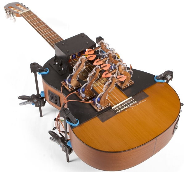
Figure 1: Professor Plucky, prototype guitar plucking robot, with six kinetic plucking mechanisms mounted between the sound-hole and bridge, and a control plucking mechanism housed in a black box spanning the neck.
