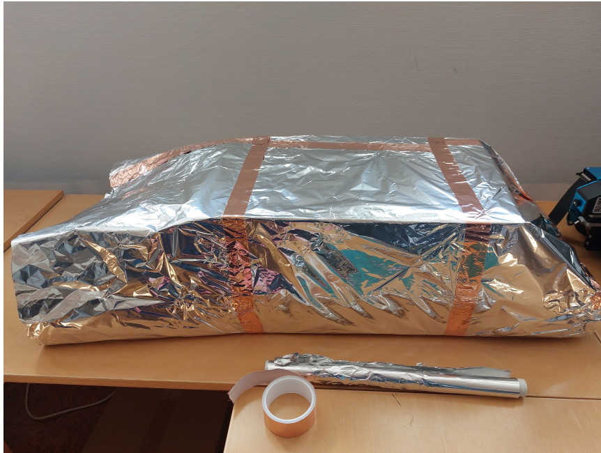
Figure 5.7: Wheeler's cap was constructed with aluminium foil, copper tape and cardboard
