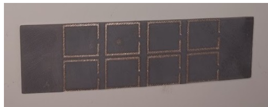
Figure 6.7: Metamaterial sheet manufactured with resonators
