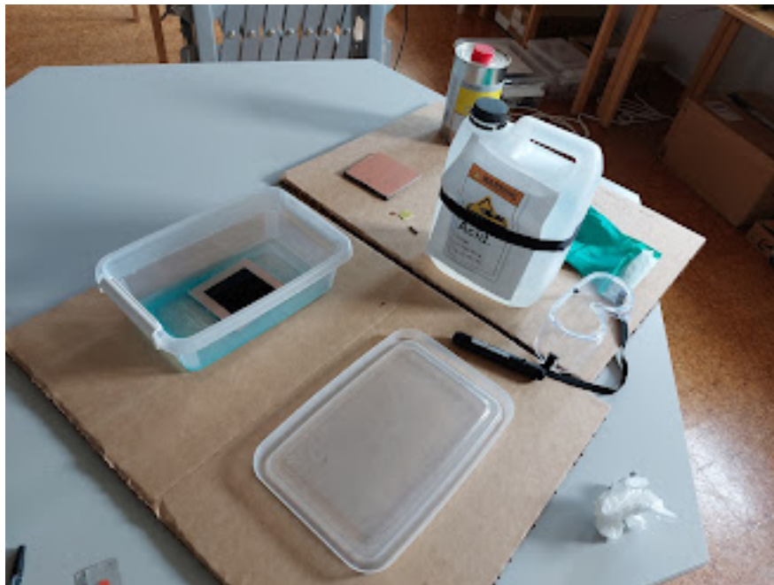
Figure 5.5: Etching with sodium persulfate
