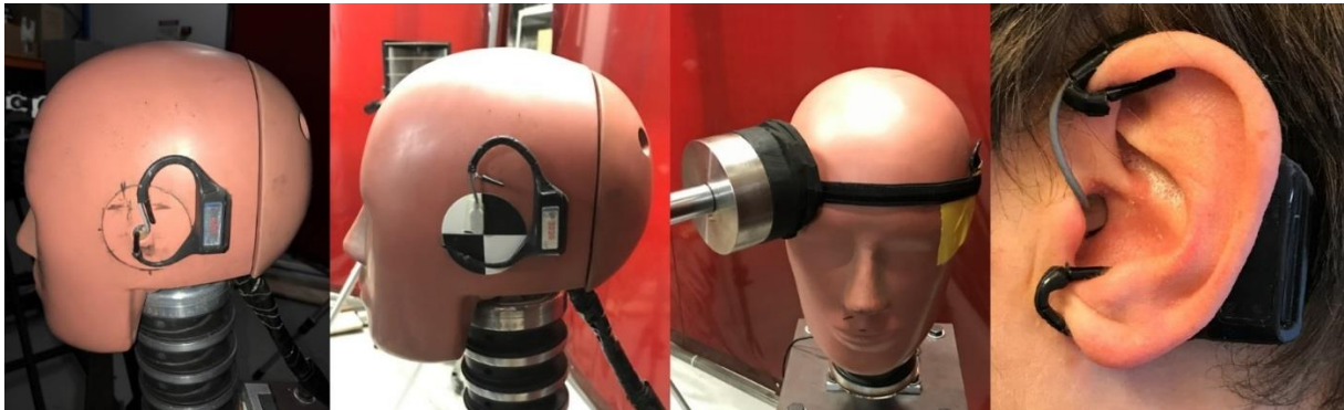
117 118 Figure 1. Mounting of the MV1 in-ear (left) and MV1 flat (left middle) on the Hybrid III 119 headform, and an example of a setup for right frontal impacts with the padded impactor 120 striking from a 45 degree angle (right middle). Shown to the right is a photo of the MV1 in a 121 real-life setup.
