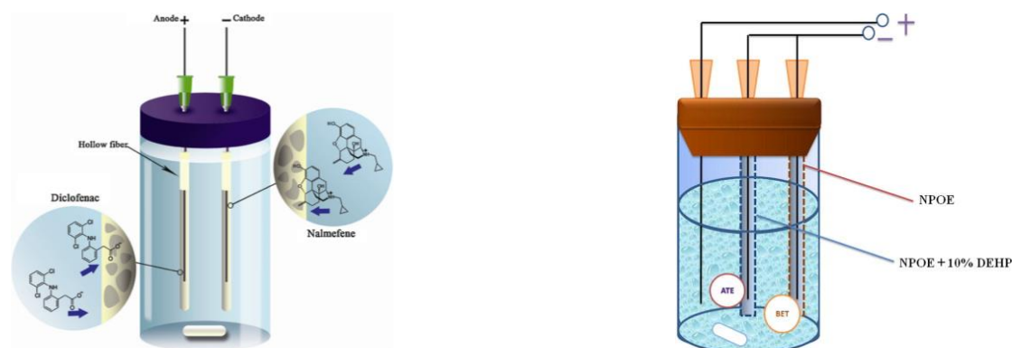
Figure 1-7. Schematic illustration of dual EME for simultaneous extraction of basic and acidic drugs (left), and for simultaneous extraction of basic drugs with different polarities (right). Reprinted with permissions from [86] © WILEY-VCH Verlag GmbH & Co. KGaA, Weinheim (2012) and [88] © Elsevier B.V (2013), respectively.
