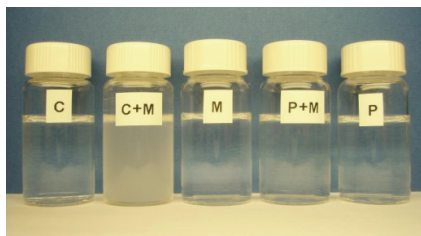
Figure 6.13 – Vials containing (C) chitosan nanoparticles, (C+M) chitosan nanoparticles mixed with mucin, (M) mucin solution, (P+M) AM-pectin nanoparticles mixed with mucin, and (P) AM-pectin nanoparticles. The samples were homogeneous without any sign of phase separation (except for sample C+M, in which particle sedimentation was observed after some minutes if left standing); the apparent turbidity increase at the bottom of the samples is merely a photographic artefact.
