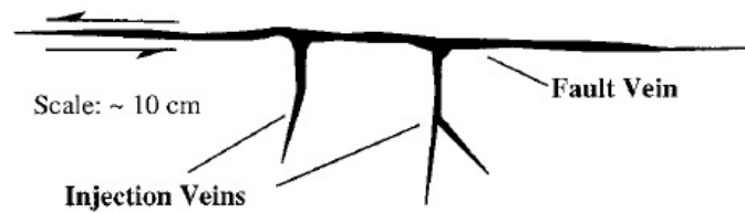
Figure 3: Schematic drawing showing the typical appearance of fault-generated pseudotachylyte. Fault-veins occur along generation surfaces with injection veins ramifying into adjacent wall rock. Both type of veins may occur several magnitudes wider or thinner, and often intertwine in complex networks. Modified from Curewitz and Karson (1999).
