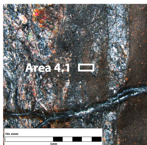
Figure 87: Micrograph in cross-polarised light of a fault vein (far right) and an adjacent fine grained wall rock zone. Area 4.1 is done over a pocket of pseudotachylyte in this zone. Image from COR-05-
