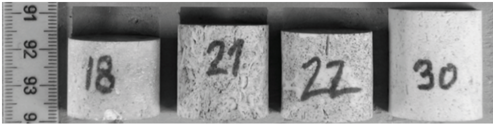
Figure 3.2: Plugs 18, 21, 22 and 30 before compaction.
