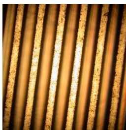
Fig. 4.3 Picture of 3D silicon structure fabricated by DRIE, 120 \mu\text{m} channels with 60 \mu\text{m} inter-channel spacing.
