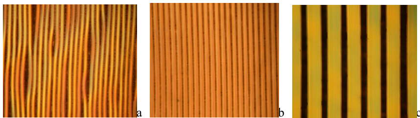
Fig. 3.4 Three different level of SU-8 lithography results from orthogonal experiments. (a) level 0, (b) level 2, (c) level 4.
